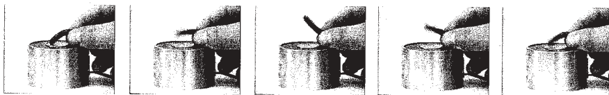
Figure 1. Snapshot of shape change of a magnetite-loaded polyvinyl alcohol hydrogel due to modulated magnetic field. The frequency of the field is 40 Hz.
